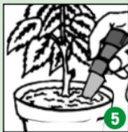
Insert the permeable BLUMAT clay tip in the earth.
